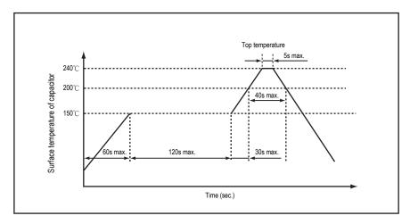
Recommended curve for lead free soldering is as following.
