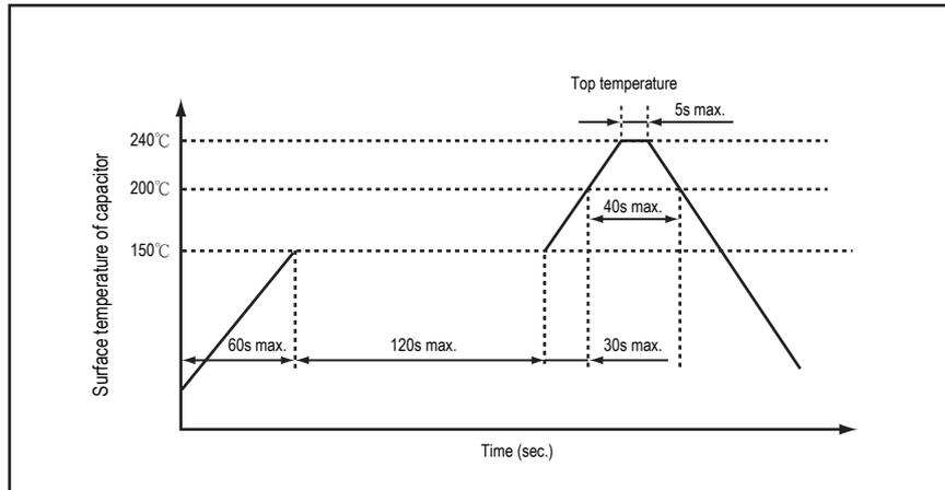
Recommended curve for lead free soldering is as following.
